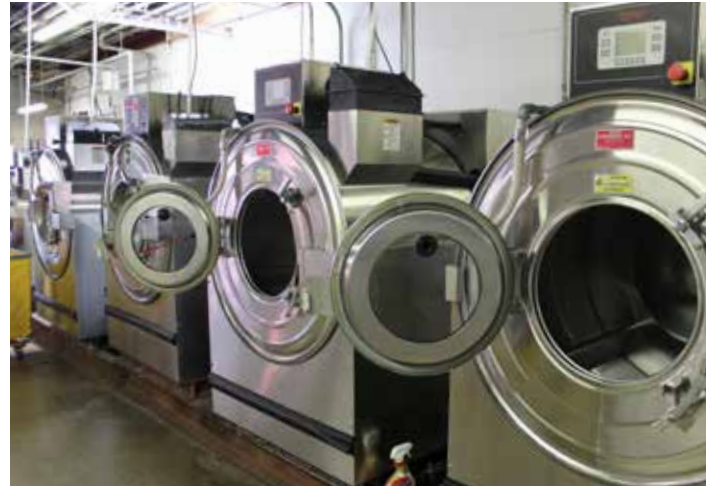
ABOVE: Tunnel washers handle high volumes of the same item, discharging to a separate unit for extraction of excess water; smaller washers handle lower volumes of single items or a wider variety and extract on their own.
