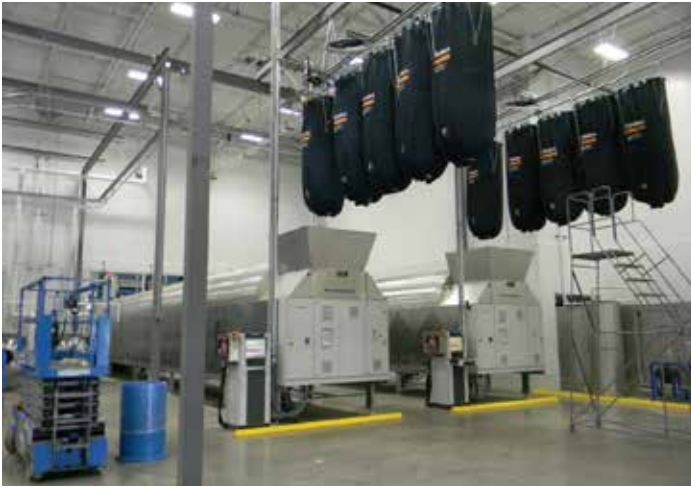
ABOVE: Tunnel washers handle high volumes of the same item, discharging to a separate unit for extraction of excess water; smaller washers handle lower volumes of single items or a wider variety and extract on their own.
