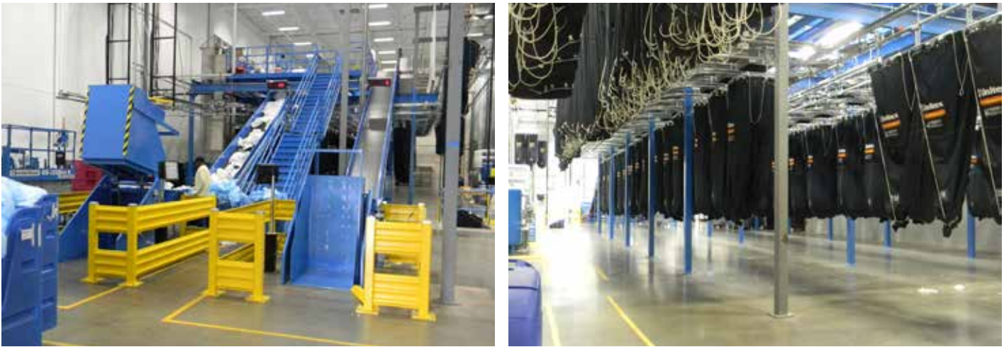
ABOVE: An automated system on a mezzanine may be used to sort items into batches of like items for washing; the system fills sling bags that are transported via rail to the wash area.
