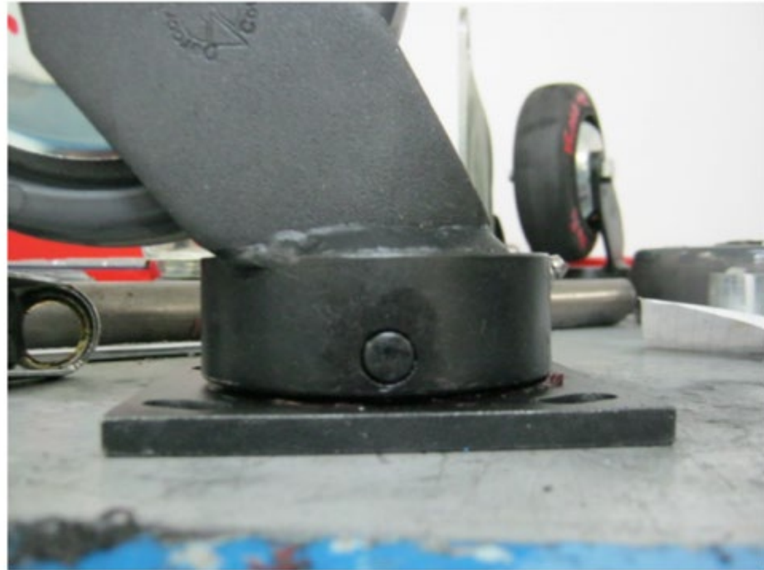
Figure. 5 – Darcor caster post endurance testing at 10,000 cycles. No damage to the swivel head.
