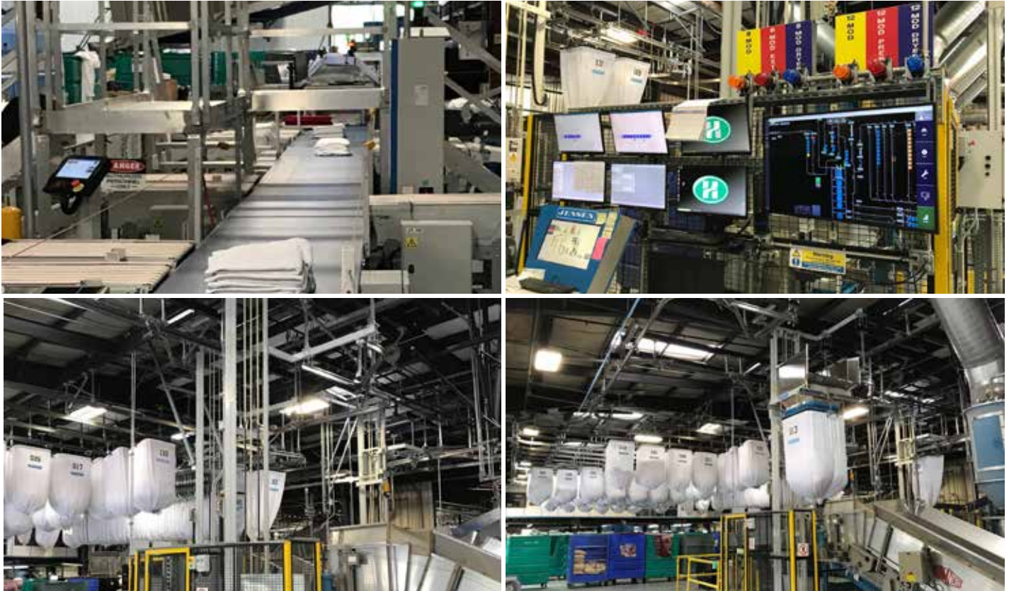
ABOVE: (from top, l/r) flatwork items move on a shuttle at the Halifax plant, which has fitted a wide range of flatwork and garment items, such as aprons, with radio frequency identification (RFID) tags. Production information is displayed on a bank of monitors. RFID tracking software helps Halifax ensure accurate deliveries. Goods move in slings to the next stage of the production process on Halifax's overhead rail system.
