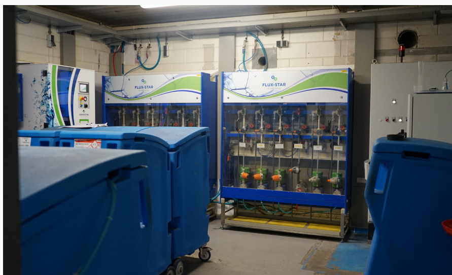
Above: (from top) a view of the plant's conventional wash aisle; employees feed garments into a sortation system; a view of the plant's chemical-injection system.
