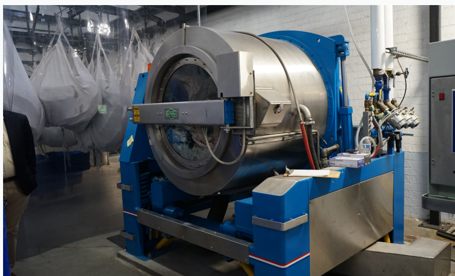
Above: (from top) Soiled goods in reusable bags hang from a ceiling rail system prior to processing; an employee adjusts settings on a vacuum system that moves goods to the next stage of processing; a washer/extractor processes stain-rewash items and other goods not processed in the tunnel washer.
